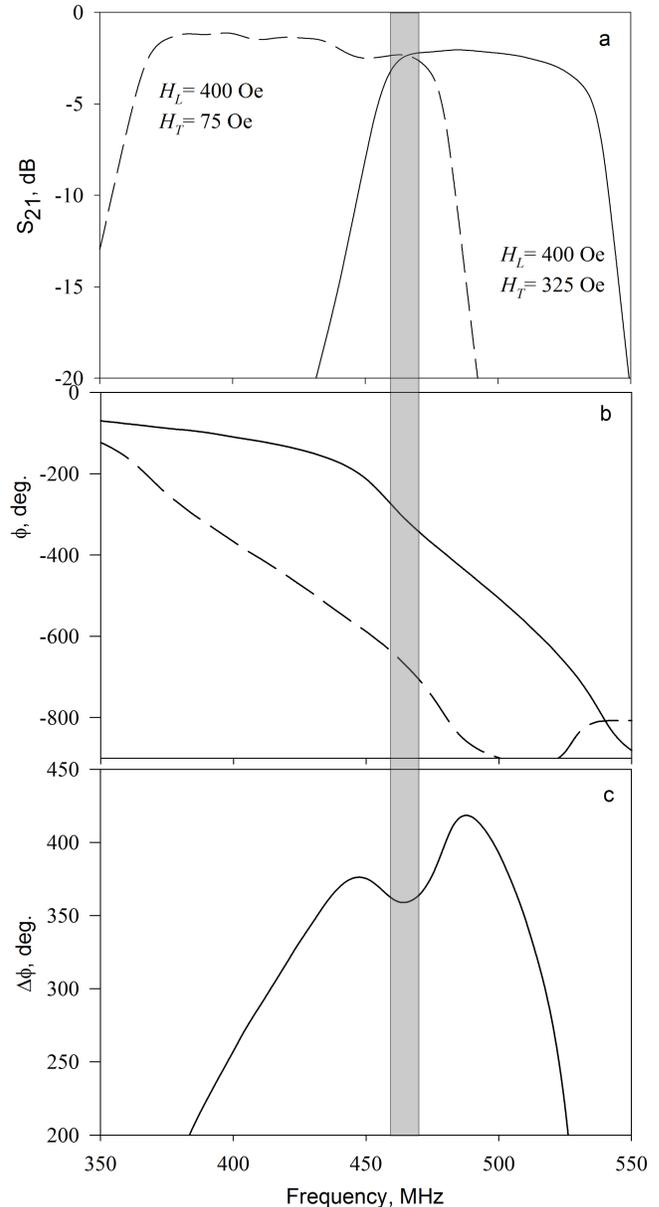
Fig. 6. (a) Frequency responses of the ferrite phase shifter for two field combinations:  $H_T = 75$  Oe,  $H_L = 400$  Oe (solid line) and  $H_T = 325$  Oe,  $H_L = 400$  Oe (dashed line). (b) Phase responses for these states. (c) Frequency dependence of the tunable phase shift corresponding to such field change. Gray area: operational band of the device.
