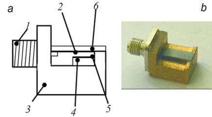
Fig. 2. (a) and (b) Measuring cell for thin film magnetic permeability characterization. 1: SMA connector. 2: inverted stripline. 3: grounded plate. 4: thin film substrate. 5: magnetic thin film. 6: alumina substrate.
