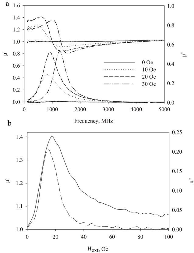
Fig. 3. (a) Frequency dependence of magnetic permeability for five-layer NiFe thin magnetic film for the various values of magnetic field (the upper curves correspond to  $\mu'$ , the lower ones to  $\mu''$ ). (b) Field dependence of magnetic permeability (solid line:  $\mu'$ , dashed line:  $\mu''$ ) measured at 500 MHz.
