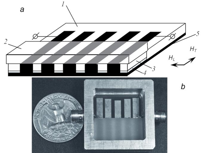
Fig. 4. (a) Structure and (b) photo of the PS. 1: microstrip substrate with high dielectric permittivity ( $\epsilon = 80$ ); 2: inverted stripline alumina substrate; 3: glass substrate of a thin film; 4: thin magnetic film; 5: grounded plate.
