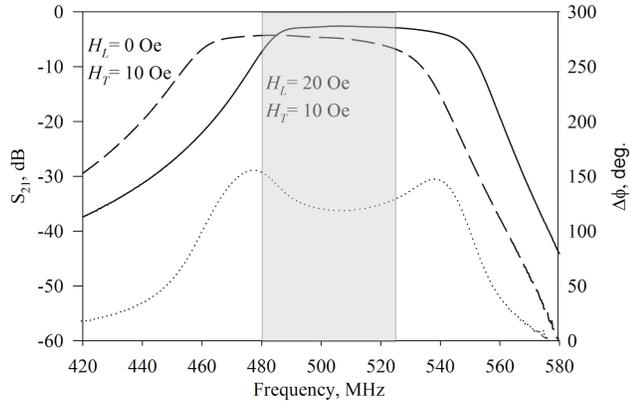
Fig. 5. Frequency responses of thin film phase shifter for two phase states corresponding to the field combination  $H_T = 10$  Oe,  $H_L = 20$  Oe (solid line), and  $H_T = 10$  Oe,  $H_L = 0$  Oe (dashed line), and frequency dependence of tunable phase shift corresponding to such field changing (dotted line).
