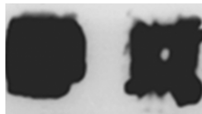
Fig. 4. Strongly defocused electron-microscopic image of spots with the left and right chiralities: the bright point at the center of the image is present for the right chirality of the spot and is absent for the left one.
