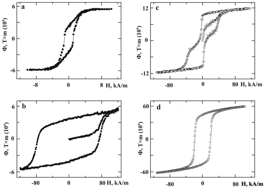
**Fig. 1** Field dependence of the magnetic moment ( $\phi$ ) of unit area of film for  $[\text{CoP}/\text{CoNiP}]_n$  films. **a** single magnetic soft layer, **b** single magnetic hard layer, **c** two-layer film ( $n = 1$ ), **d** five-layer film ( $n = 5$ ). Temperature  $T = 78$  K
