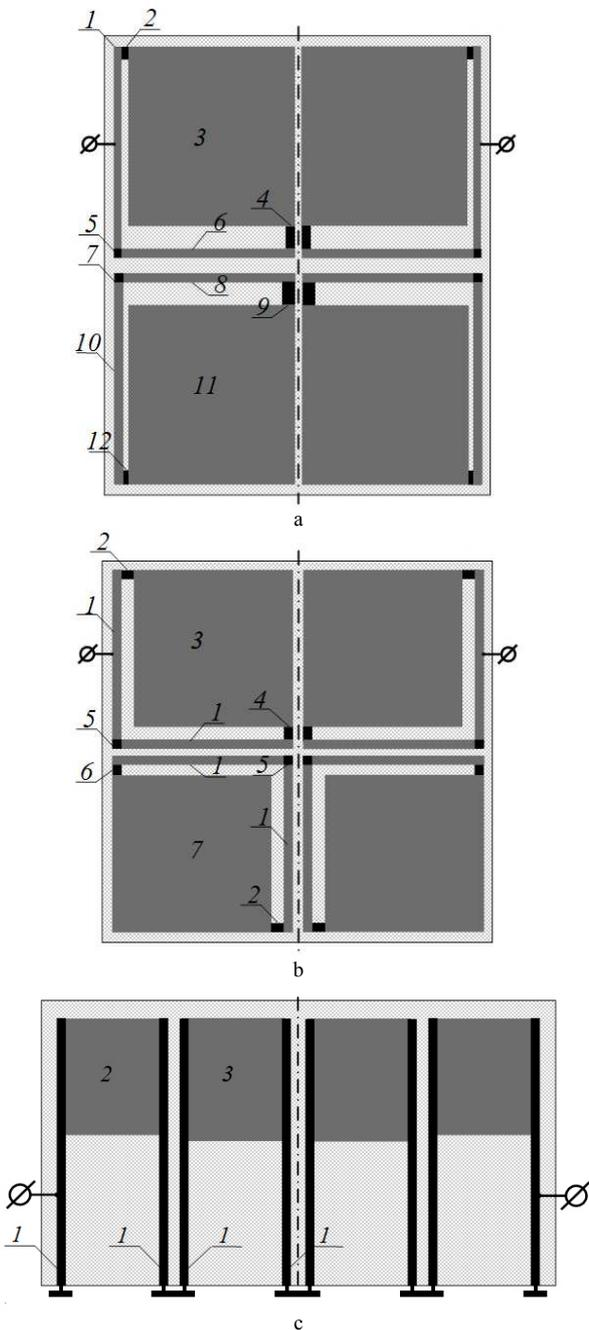
Fig. 3. Topology of the strip conductors portions of 4th order microstrip filters.
