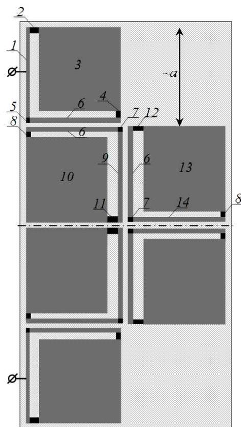
Fig. 7. Topology of the 6<sup>th</sup> order filter conductors, based on electromagnetic crystal with a defect.
