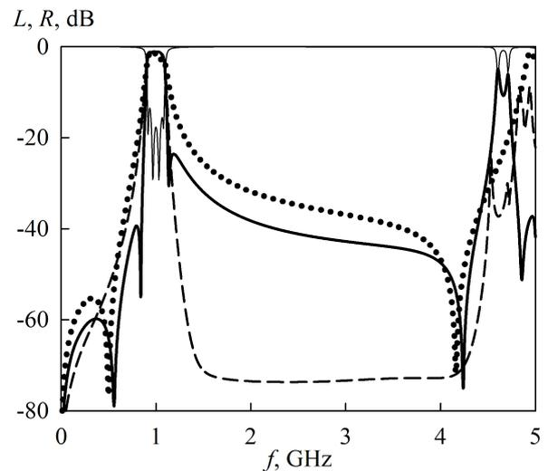
Fig. 4. Synthesized AFCs of 4<sup>th</sup> orders filters. Points – used the topology of conductors presented in Fig.3a, solid lines – in Fig.3b, dashed lines – in Fig.3c.
