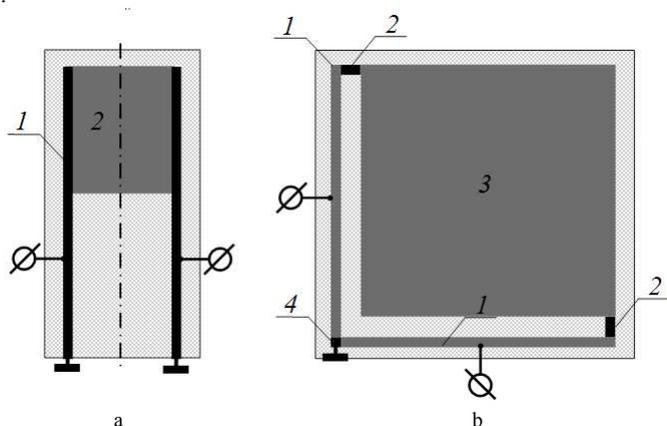
Fig. 1. Topology of the strip conductors (black or gray) of microstrip resonators with wide stop band.
