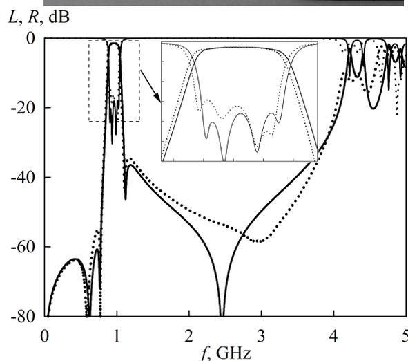
Fig. 10. AFCs of 4<sup>th</sup> order bandpass filter. Lines are the calculation, and points are the measurements. In the insets we show the photograph of fabricated sample.
