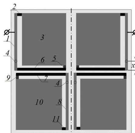
Fig. 9. Topology of the strip conductors of experimental filter.
