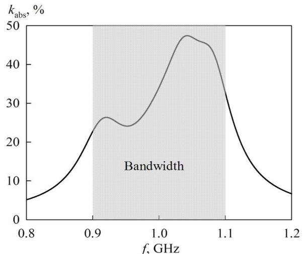
Fig. 5. The frequency dependence of absorption coefficient calculated in the narrow band for the filter with the topology of conductors presented in Fig.3a.
