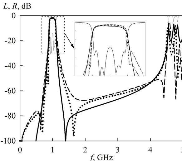
Fig. 8. Synthesized AFCs of 6<sup>th</sup> orders filters. Dashed lines – used the topology of conductors presented in Fig.6a, solid lines– in Fig.6b, points – in Fig.7.
