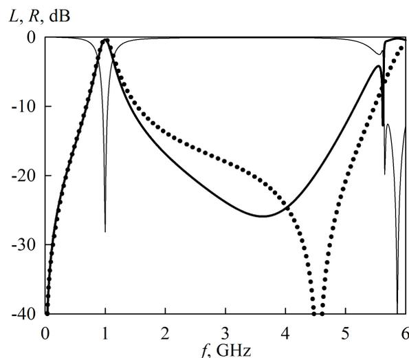
Fig. 2. AFCs of the initial resonator (points) and transformed resonator (lines).
