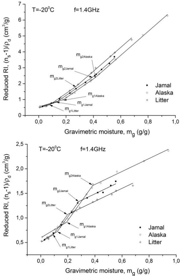
Fig. 1 Behavior of the reduced RI,  $(n_s - 1)/\rho_d$  vs. gravimetric moisture at the temperatures of  $20^\circ\text{C}$  and  $-20^\circ\text{C}$  and the wave frequency of  $1.4$  GHz for different organic soils. The RI dependences on soil moisture are piecewise linear functions in certain moisture ranges, indicating contributions of particular forms of soil water. The solid lines show the fits of formula (2) of [2] to the measured data, which are shown by symbols.
