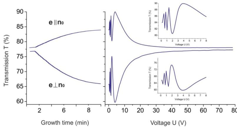
Fig. 3. Regimes of variation in optical transmission  $T$  of the 5CB domain formed by the PC surface with time  $t$  (on the left) and electric voltage  $U$  applied to the domain (on the right): the polarization vector  $e$  is parallel (on the top) and perpendicular (in the bottom) to the nematic direction  $n_0$ . Insets: enlarged portions of the  $T(U)$  dependences.
