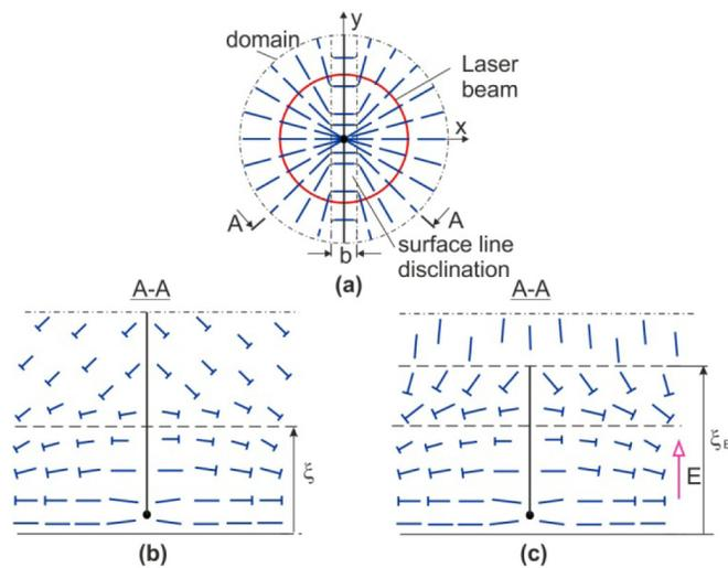
Fig. 4. LC director field distribution in the domain formed by the PC surface. (a) In the  $xy$  plane at the distance  $z > \xi$  from the PC film surface. (b) In the A-A cross section in zero external field. (c) In external field  $E$ .
