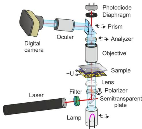
Fig. 1. Experimental setup for determining the transmission of light passing through the nematic domain formed by the polycarbonate film.
