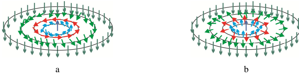
Figure 1. Magnetic skyrmion textures: a) Bloch ( \varphi ) skyrmion (magnetization rotates in the plane perpendicular to the radial direction), b) Neel ( \rho ) skyrmion (magnetization rotates along the in-plane radial direction).
