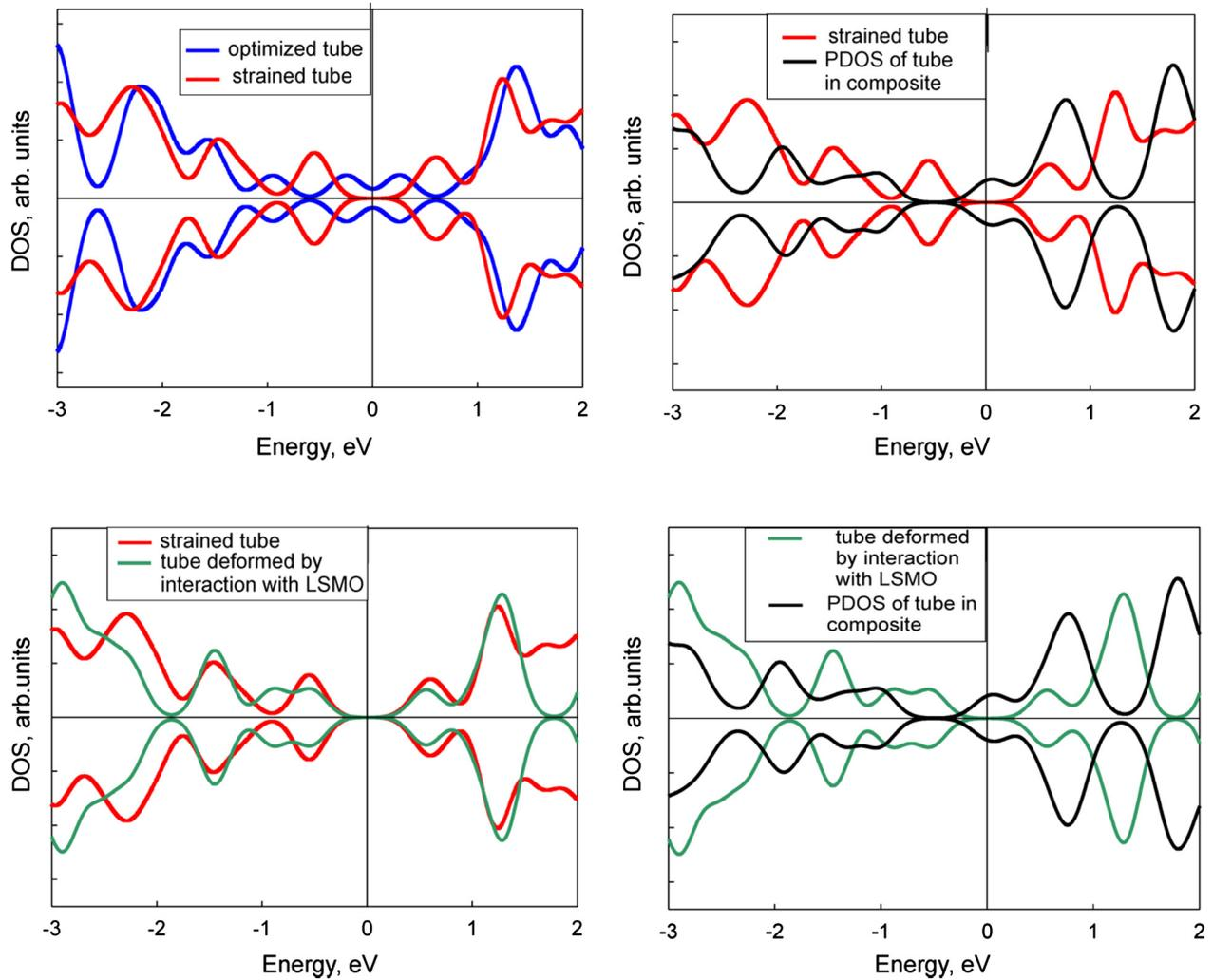
**Fig. 6.** Densities of states for CNT(5,5) Blue, red, green and black lines correspond to the relaxed CNT's structure, strained CNT structure with LSMO translation vector adopted, freestanding CNT at the same geometry as in the composite, and partial density of states the nanotube in CNT/LSMO(Sr-O) composite, respectively. (For interpretation of the references to colour in this figure legend, the reader is referred to the web version of this article.)
