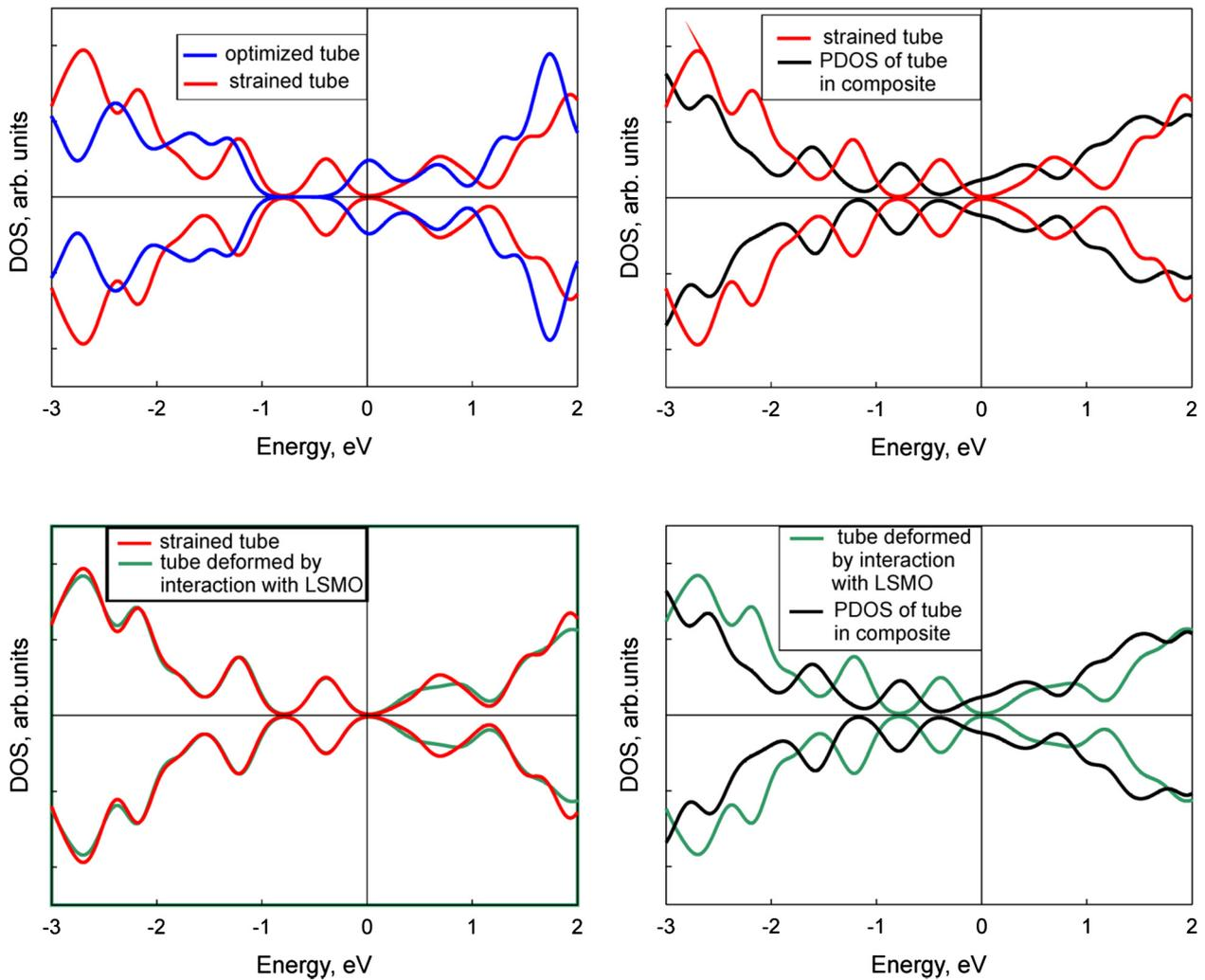
**Fig. 5.** Densities of states for CNT(9,0). Blue, red, green and black lines correspond to the relaxed CNT's structure, strained CNT structure with LSMO translation vector adopted, freestanding CNT at the same geometry as in the composite, and partial density of states the nanotube in CNT/LSMO(Sr-O) composite, respectively. (For interpretation of the references to colour in this figure legend, the reader is referred to the web version of this article.)
