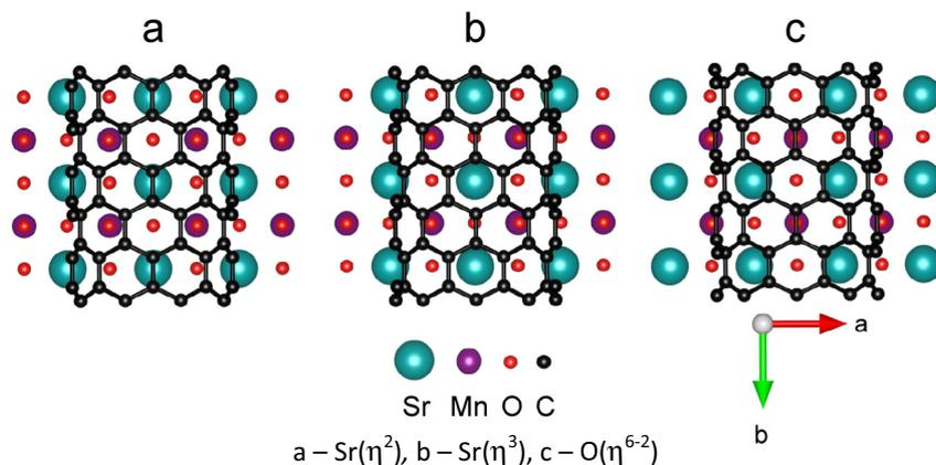
**Fig. 2.** Different configurations of CNT(9,0)/LSMO(Sr-O) nanocomposites. For the sake of better representation, the upper part of tubes is cut.
