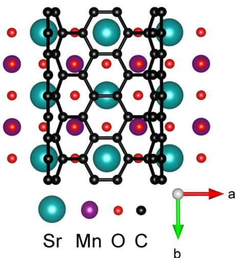
**Fig. 3.** Structure of CNT(5,5)/LSMO(Sr-O) nanocomposite. For the sake of better representation, the upper part of the tube is cut.
