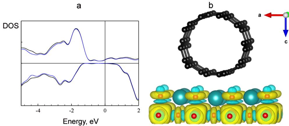
**Fig. 4.** (a) Density of states of CNT(9,0)/LSMO(Sr-O) heterostructure. Black and blue lines correspond to the total and partial LSMO DOSes, respectively. (b) Spatial distribution of spin density in CNT(5,5)/LSMO(Sr-O) heterostructure. Yellow and blue areas correspond to spin-up and spin-down density, respectively. (For interpretation of the references to colour in this figure legend, the reader is referred to the web version of this article.)
