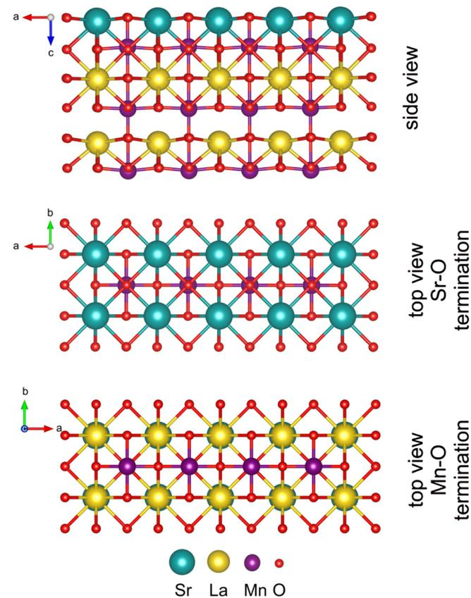
Fig. 1. Top and side views of Mn-O and Sr-O terminated LSMO slab.
