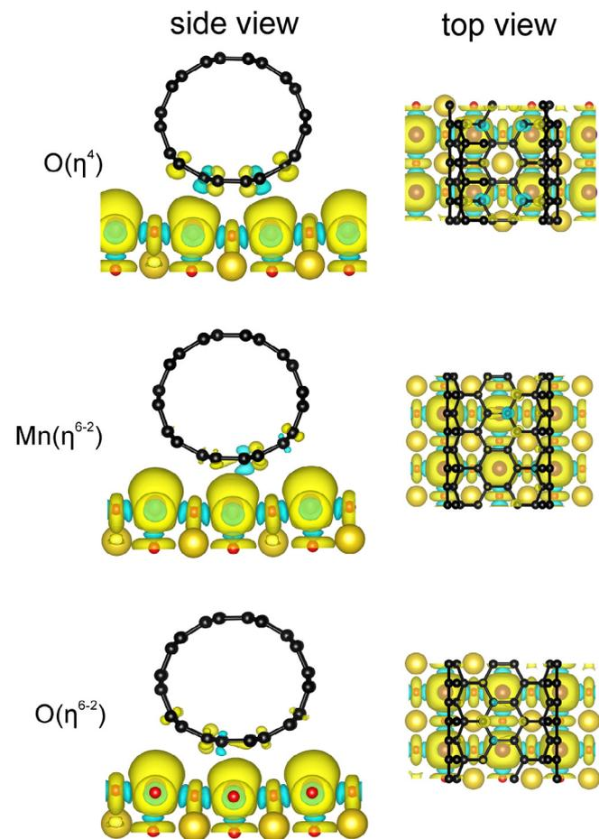
**Fig. 8.** Spatial spin density distribution in CNT(5,5)/LSMO(Mn-O) nanocomposites. Yellow and blue areas correspond to spin-up and spin-down density, respectively. (For interpretation of the references to colour in this figure legend, the reader is referred to the web version of this article.)
