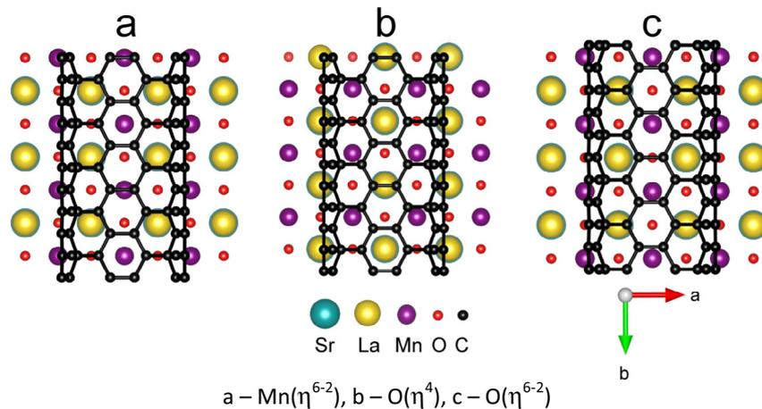
**Fig. 7.** (a) Mn( $\eta^{6-2}$ ), (b) O( $\eta^4$ ) and O( $\eta^{6-2}$ ) CNT(5,5)/LSMO(Mn-O) configurations. For the sake of better representation, the upper part of the tube was cut.
