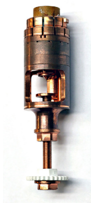
Fig. 1. Measurement cell for thermal expansion, magnetostriction and piezoelectric effect measure.
