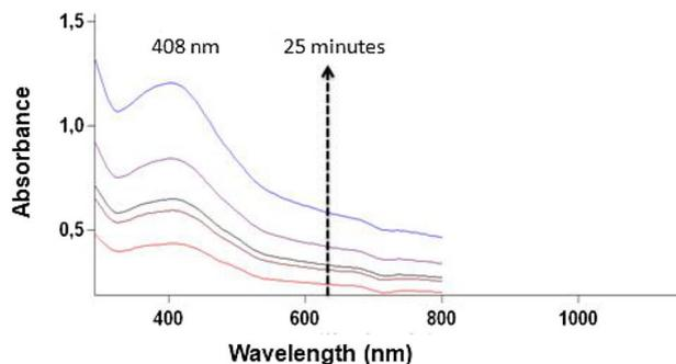
Fig. 1 UV–visible spectrum of silver nanobactericides
