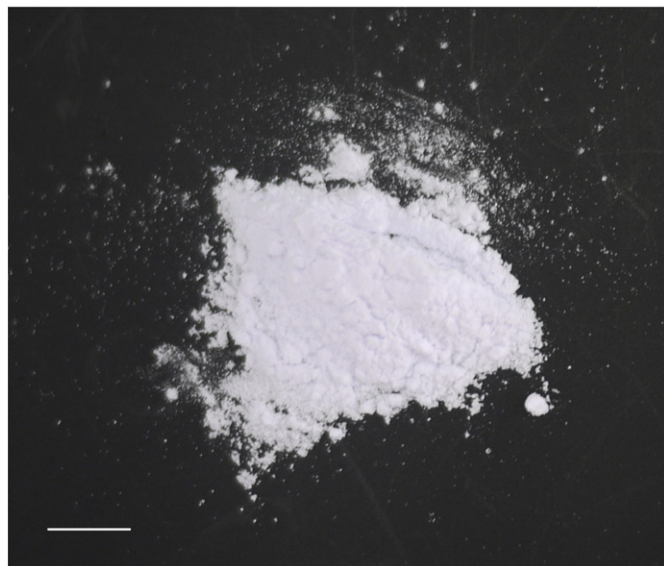
Fig. 4. The digital image of \text{Rb}_3\text{EuB}_6\text{O}_{12} powder under illumination by white light. The length of the scale bar is 7 mm.
