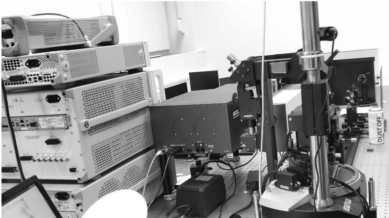
*Fig 1. Complex for nanoscale researches with TERS, SNOM, BLS, XPM*
