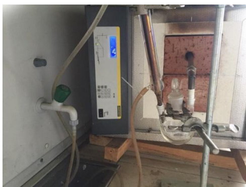
Fig. Laboratory coke unit
