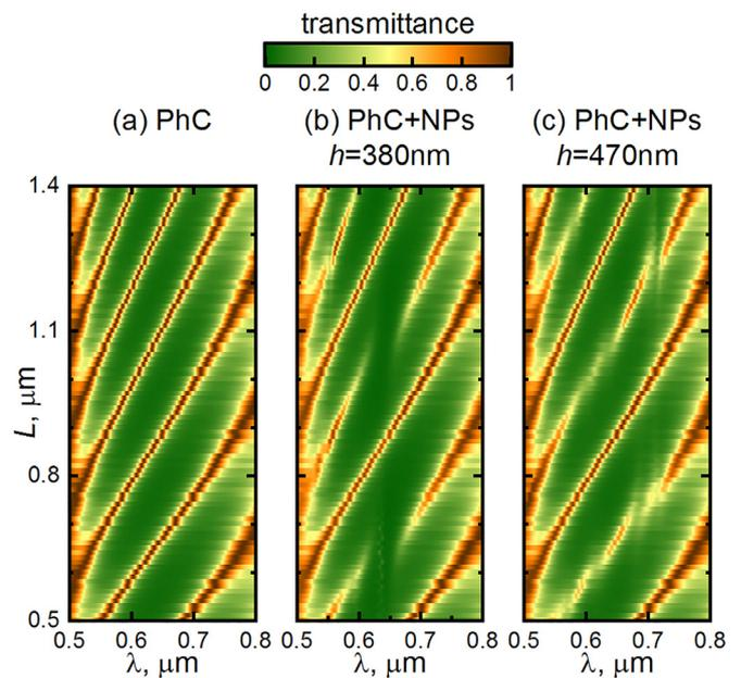
**Fig. 6.** Transmittance of (a) PhC without NPs; and PhC with array of NPs embedded in the middle of its defect layer for two periods  $h$ : (b) 380 nm, and (c) 470 nm.
