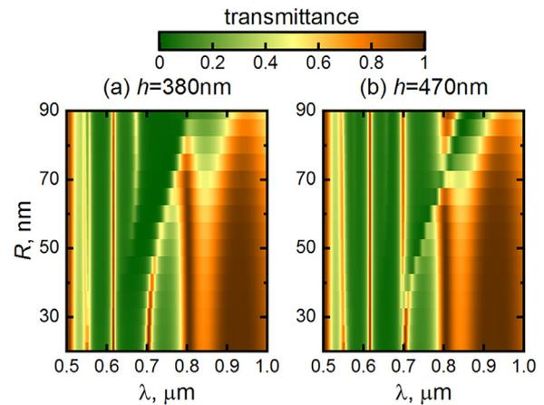
**Fig. 5.** Transmittance of 2D lattice of NPs with (a)  $h = 380$  nm and (b)  $h = 470$  nm embedded in the middle of the defect layer of PhC with  $L = 1230$  nm.
