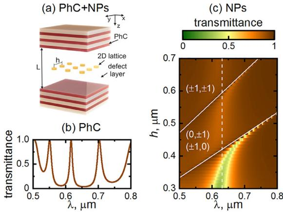
**Fig. 1.** (a) Schematic representation of PhC and 2D array of NPs embedded in its defect layer; (b) Transmittance of bare PhC with  $L = 1230$  nm; (c) Transmittance of 2D lattice of Au nanodisks with height  $H = 50$  nm and radius  $R = 40$  nm embedded in homogeneous environment with  $\varepsilon_{\text{def}} = 2.25$ . Solid lines represent Wood-Rayleigh anomalies of  $(p, q)$  order, while vertical dashed line indicates the position of dipolar LSPR of the isolated NP.
