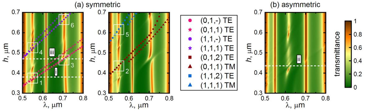
**Fig. 2.** Transmittance of 2D array of gold nanodisks embedded in PhC defect layer: (a) in the middle, and (b) shifted along  $z$  axis by 100 nm. Symbols denote Wood–Rayleigh anomalies of  $(p, q, s)$  order for TE and TM polarization. Note that for the convenience of the Reader, only position of strongly coupled Wood–Rayleigh anomalies are shown.
