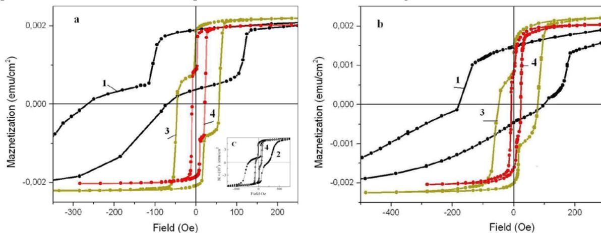
**Figure 3.** Magnetization loops for CoNi (25 nm) / Si / FeNi (25 nm) / Si films. a, b –  $t_{Si}$  = 2; 7 nm, inset c – CoNi (53 nm) / Si (2 nm) / FeNi (72 nm) films, 1, 2, 3, 4 –  $T$  = 5, 40, 100, 300 K.
