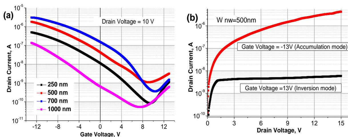
**Figure 2(a, b).** (a) The transfer characteristics  $\text{Co}_2\text{FeSi/SOI}$  back-gate nanowire transistor with a channel width of width of 250 nm to 1000 nm plotted on a semilog scale at different voltages on source-drain; (b) Output characteristics device in inversion and accumulation mode with a channel width of 500 nm.
