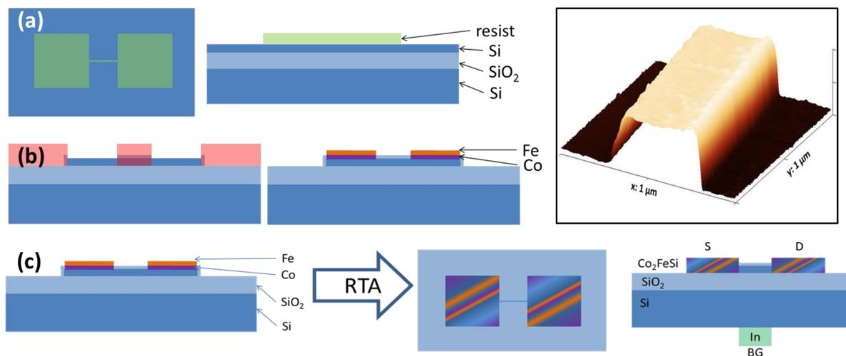
**Figure 1(a, b, c)** The main technological stages of the formation of devices (a) - (c). Inset: AFM image of a 500 nm wide device.
