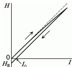
**Figure 5.** The dependence of the magnetic field of a superconducting solenoid from the electric current flowing through the coil.
