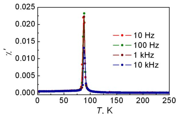
**Figure 2.** Temperature dependences of  $\text{Cu}_2\text{MnBO}_5$  AC magnetic susceptibility.
