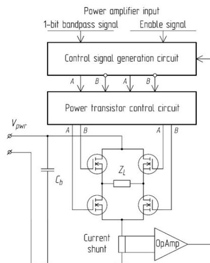
Fig. 2. The power amplifier block diagram.
