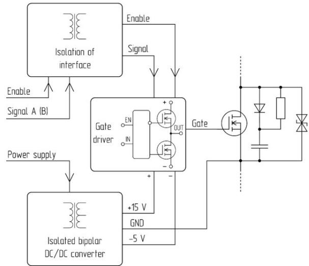
Fig. 4. The part of the power transistor control circuit (for one power transistor).
