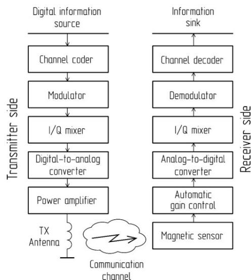
Fig. 1. Near-field magnetic communication system block diagram.
