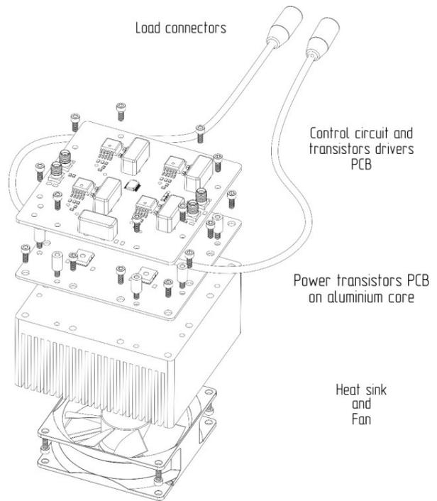
Fig. 5. The power amplifier construction.
