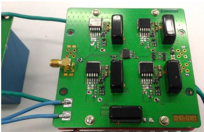
Fig. 6. The power amplifier prototype.
