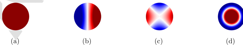
FIG. 2. (Color online) Profiles of propagating modes in the cylindrical waveguide. (a) In channel 1 with cut-off frequency \omega = 0 and indices p = 0, q = 1 ; (b) in channels 2 and 3 with cut-off frequency \omega = 1.8412 and indices p = \pm 1, q = 1 ; (c) in channels 4 and 5 with cut-off frequency \omega = 3.0542 and indices p = \pm 2, q = 1 ; (d) in channel 6 with cut-off frequency \omega = 3.8317 and indices p = \pm 0, q = 2 .
