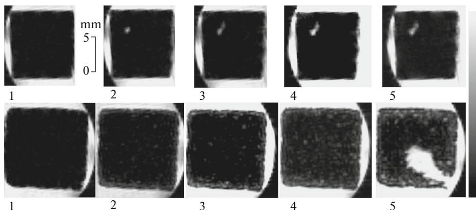
**Fig. 3.** Upper row: tomographic images of the TZMK + PPU-90 specimen within (1) 5 min, (2) 24, (3) 120, (4) 192, and (5) 312 h after dipping into water. Lower row: tomographic images of the VTI + PPU-90 specimen within (1) 5 min, (2) 120, (3) 192, (4) 312, and (5) 456 h after dipping into water. The cross section of a tomographic slice with a thickness of 1 mm relative to the geometry of the specimen is analogous to that shown in Fig. 1.
