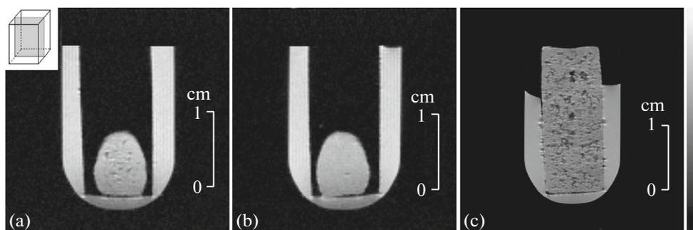
**Fig. 2.** Tomographic images of the TZMK specimen within (a) 5 min and (b) 14 days after the second dipping into water and (c) a specimen subjected to preliminary heating. The cross section of a tomographic slice with a thickness of 1 mm relative to the geometry of the specimen is shown.
