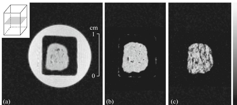
**Fig. 1.** Tomographic images of the TZMK specimen (a) after 2-h exposure to water, (b) immediately after removal from water, and (c) after 24 h of exposure to open air. The cross section of a tomographic slice with a thickness of (a) 1 and (b, c) 0.5 mm relative to the geometry of the specimen is shown.
