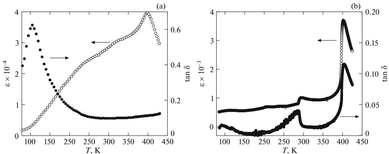
**Fig. 3.** Temperature dependences of the permittivity and dissipation factor for (a) the BaTiO<sub>3</sub> nano- and (b) microceramics.
