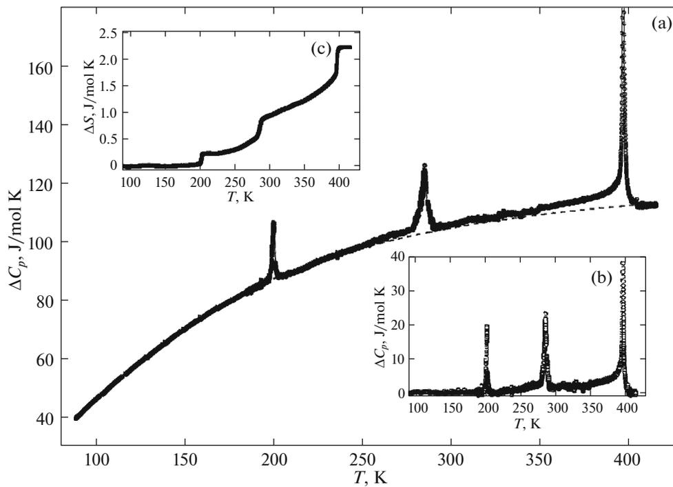
Fig. 6. Temperature dependences of (a) the specific heat, (b) excess specific heat, and (c) entropy for mBT.
