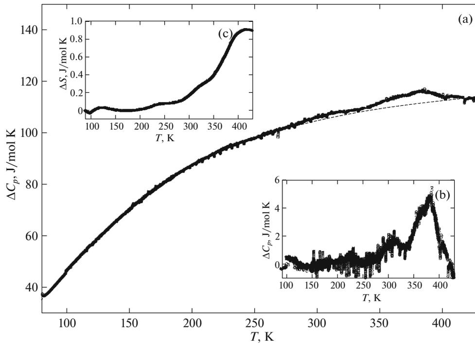
Fig. 5. Temperature dependences of (a) the specific heat, (b) excess specific heat, and (c) entropy for nBT.
