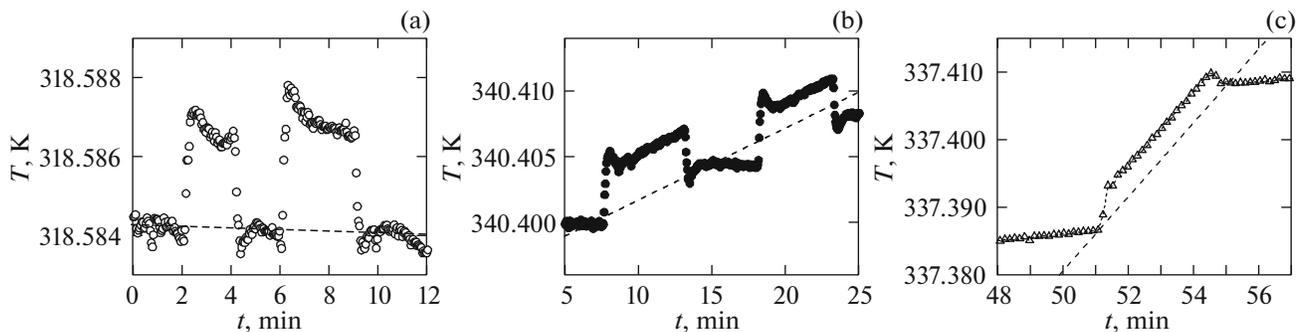
**Fig. 8.** Temperature behavior variation in an applied electric field as a result of the intensive electrocaloric effect at temperatures of about (a) 320 and (b) 340 K for nBT (2 kV/cm) and (c) 340 K for mBT (2.5 kV/cm).
