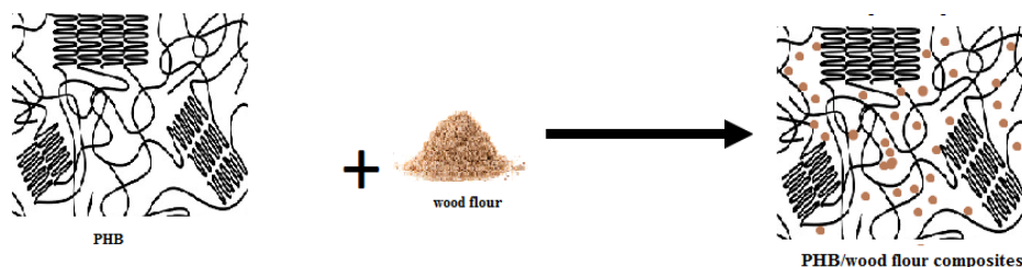
Fig. 4. Schematic representation of the original polymer, wood flour, and P(3HB)/wood flour composites
