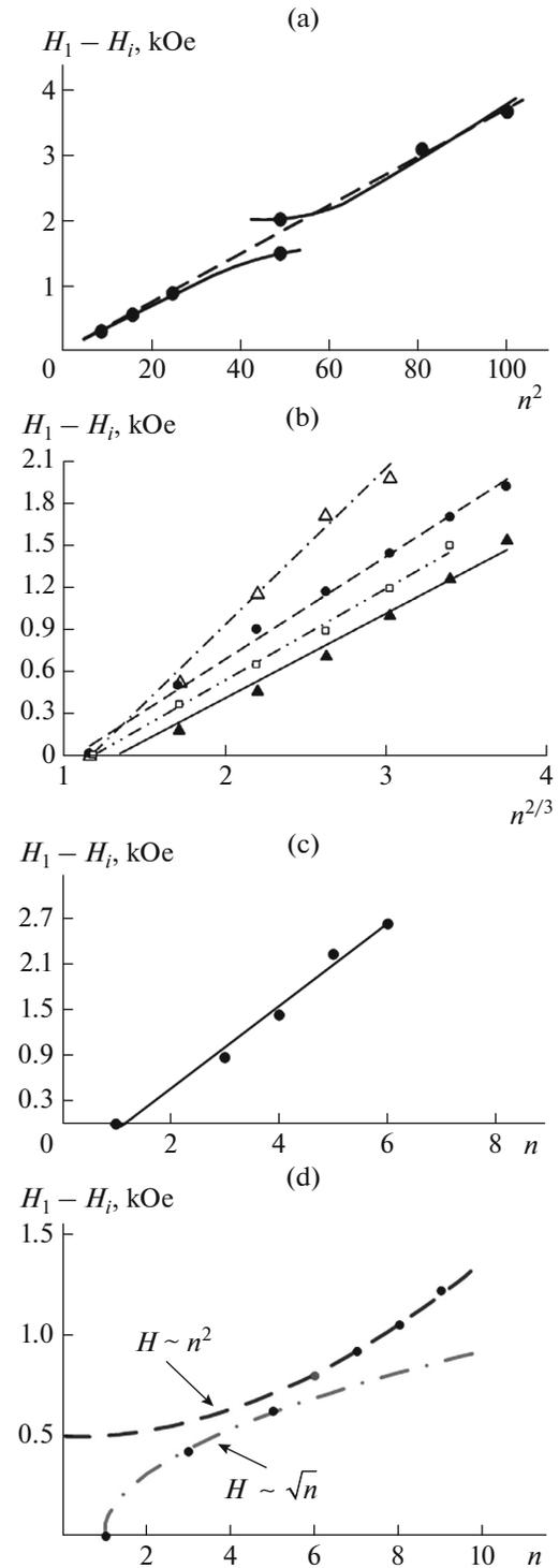
**Fig. 2.** Dependences of resonance fields on mode number for (a, b) Co-P and (c, d) Co-Ni planar systems.
