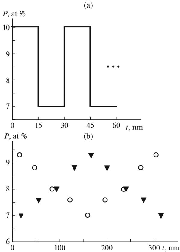
**Fig. 1.** Exchange coupling constant distribution that results in the formation of (a) the first stop band of the magnon crystal or (b) the dependence of the resonance fields  $H_r(n) \sim n^{2/3}$ .
