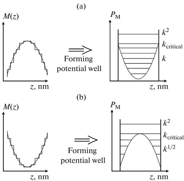
**Fig. 3.** Functional dependence of magnetization  $M$  over the layered coating thickness and the profile of magnetic potential  $P_M$  for the Co–Ni planar coatings
