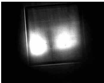
Fig. 2. Optical image of luminescence area inside 3rd milled square with 428 milled depth.
