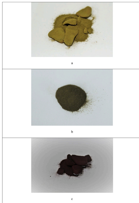
Fig. 1. Photo of (a) \text{BaDyCuS}_3 , (b) \text{BaHoCuS}_3 and (c) \text{BaYbCuS}_3 products.
