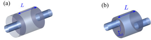
Figure 19. Cylindrical resonator with (a) a coaxially and (b) a non-coaxially attached non-axisymmetric cylindrical waveguide. The input waveguide can freely move along the resonator axis and rotate about the symmetry axis of the resonator. Reprinted from [141], Copyright (2018), with permission from Elsevier.
