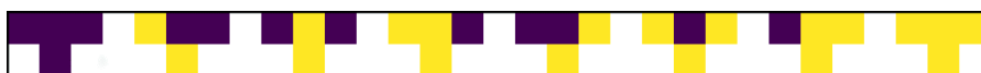
Figure 1. Ones are colored in yellow and zeros, in purple. The three upper cells will be called the neighbourhood. The figure illustrates rule (0, 1, 1, 1, 1, 1, 1, 1) equal to 254 in decimal notation.
