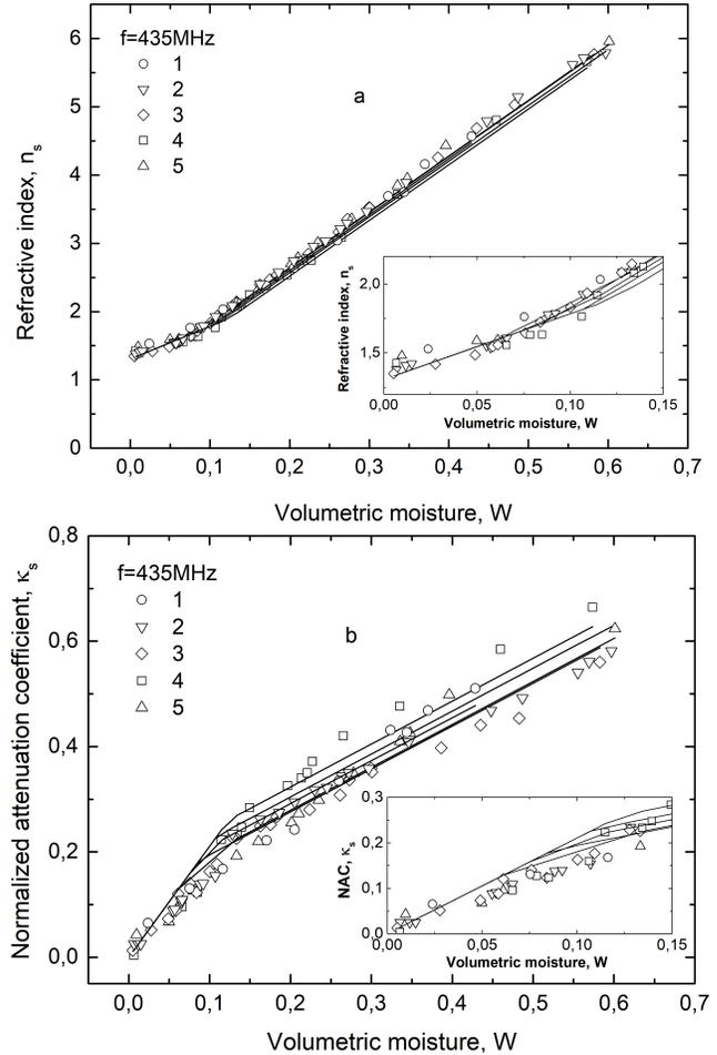
Fig. 1. Dependencies of (a) RI and (b) NAC from moisture measured in the experiment (symbols) and calculated based on model (solid lines)
