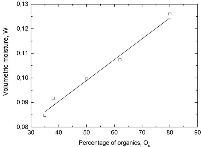
Fig. 2. Dependence of the maximum of bound water  $W_t$  on the content of organic matter in the soil  $O_s$  (symbols) and linear approximation (solid line).  $W_t = 0.059 + 8.146 \cdot 10^{-4} O_s$ .
