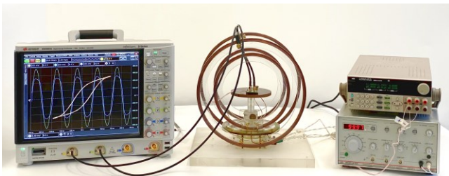
Fig. 2. Measuring unit for the observation of hysteresis loops in thin ferromagnetic films
