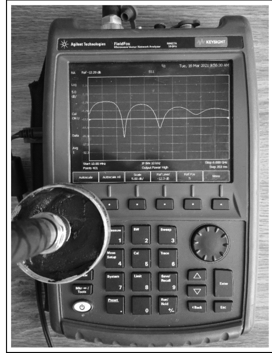
Figure 2. The process of measuring CP spectrums by the probe placed into plastic cap using VNA.
