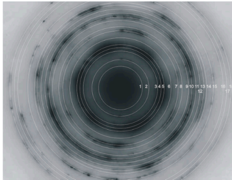
Figure 3. The electron diffraction pattern of the \text{Ni}_{50.6}\text{Ti}_{49.4} alloy, coarse-grained after tension.
