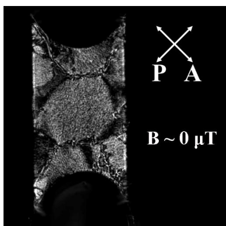
Figure 1: Magnetic domains in a ferromagnetic nematic suspension of BHF NPLs.
