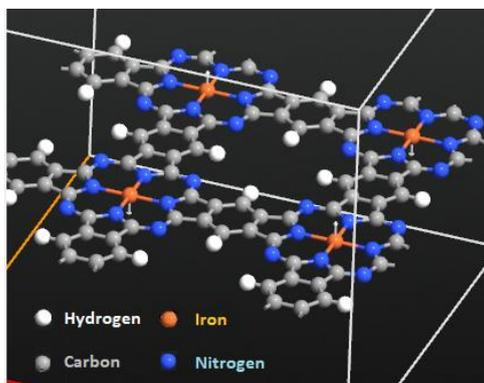
Fig. 1. Supercell of the FePPC with anti-ferromagnetic coupling of Fe atoms.
