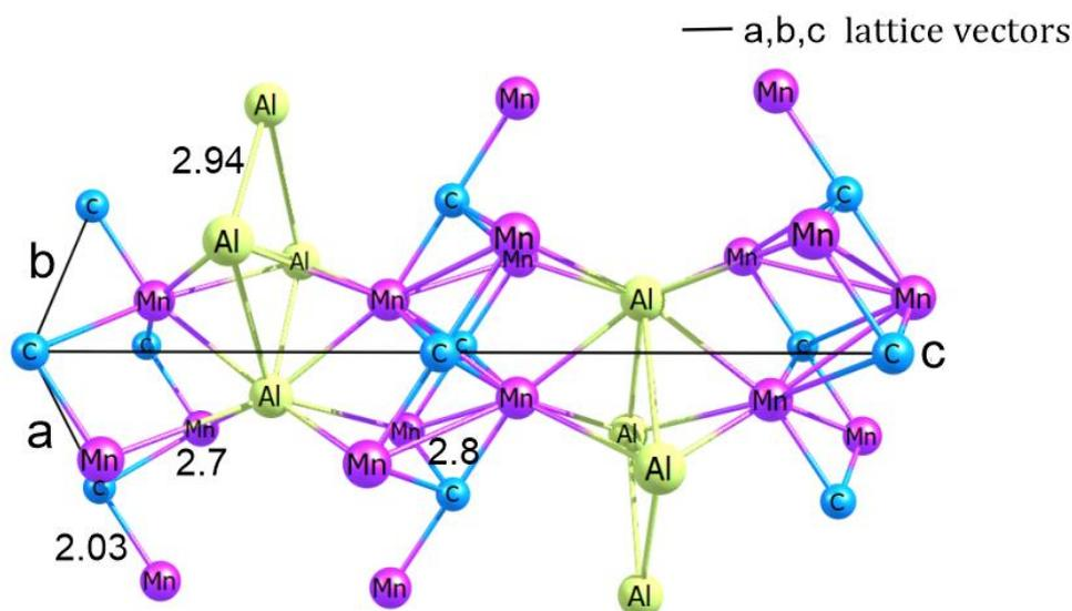
Figure 1. Atomic structure of Mn<sub>2</sub>AlC. The cell parameters:  $a = 2.94 \text{ \AA}$ ;  $b = 2.94 \text{ \AA}$ ;  $c = 12.87 \text{ \AA}$
