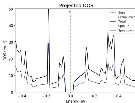
Fig. 2. Non-conductive gap on Fermi level of the pDOS for the antiferromagnetic configuration.
