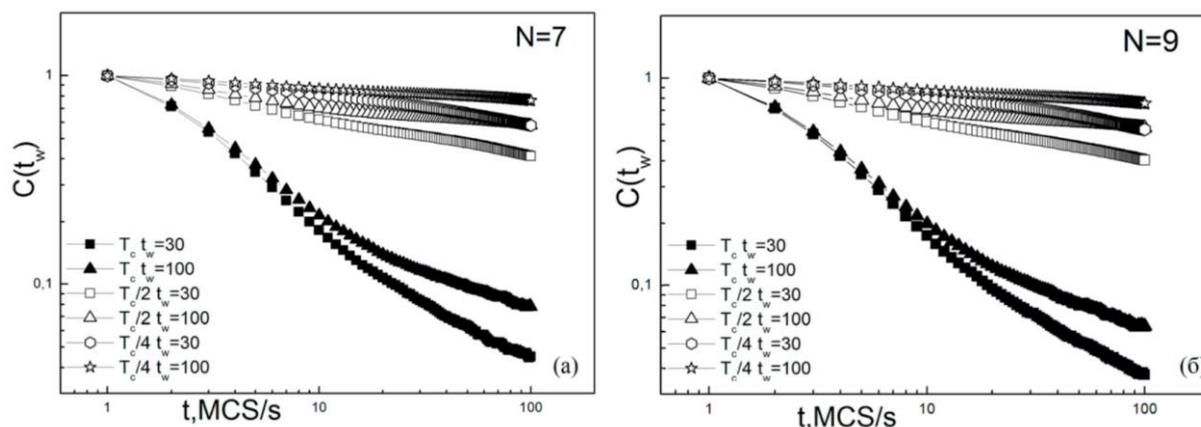
Figure 1 - Dependence  $C(t, t_w)$  at  $t_w = 30; 50; 100$  at  $N = 7$  (a) and  $N = 9$  (b). The measurements were carried out at the critical temperature  $T_c$  and at  $1/2$  of  $T_c$ .
