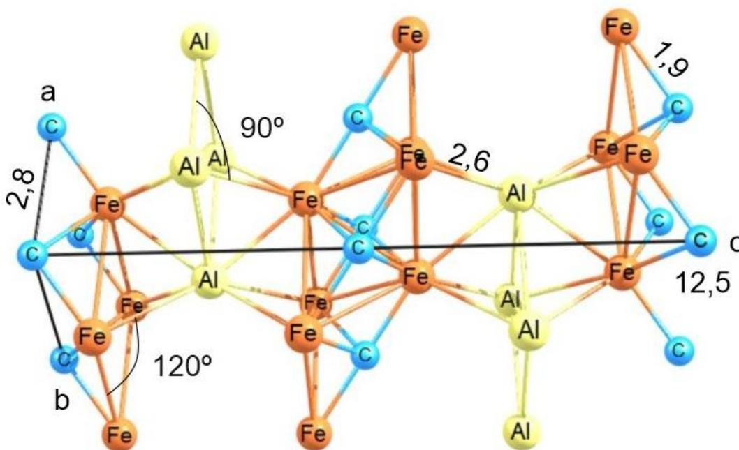
Figure 1. Structure of Fe<sub>2</sub>AlC phase calculated by B3LYP/DZVP
