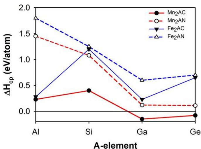
Figure 1. Calculated formation enthalpies of  $M_2AX$  phases with respect to most competing phases in dependence on the composition of M-, A- and X-sites.
