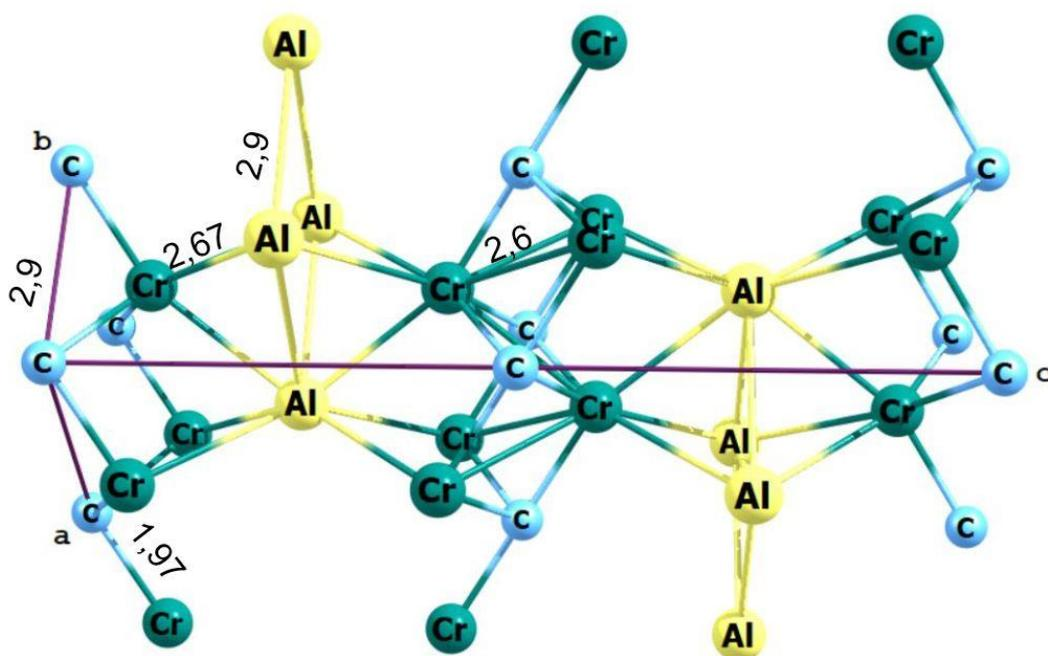
Figure 1. Structure of MAX-phase Cr<sub>2</sub>AlC with space group P6<sub>3</sub>/mmc, cell parameters a=2.9Å, b=2.9Å, c=12.46Å. a, b, c - lattice vectors.
