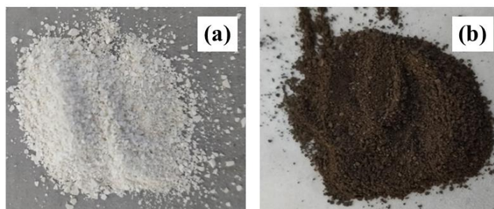
Fig. 1 Morphology of (a) ZnO NPs and (b) Ag/ZnO NPs synthesis by using Caulerpa racemosa extract
