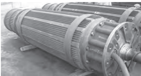
Fig. 1 A submersible motor with large ratio of diameter to shaft length.
