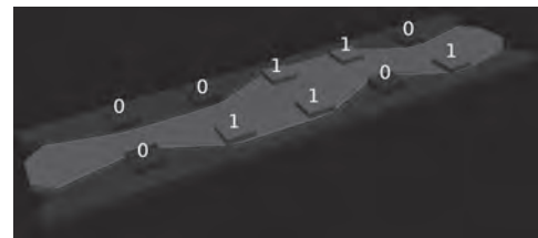
Fig. 2. Concept of DW-based AFM memory with bits defined by the direction of the Neel order parameter at the mesa top surface (red or blue color, respectively).
