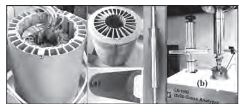
Fig. 5 The prototype of 200 kW high-speed generator and the experimental setup to measure the magnetic flux density distribution on the rotor core: (a) Stator core with the winding, Permanent magnet, and assembled rotor core; (b) the experimental setup to measure the rotor core.
