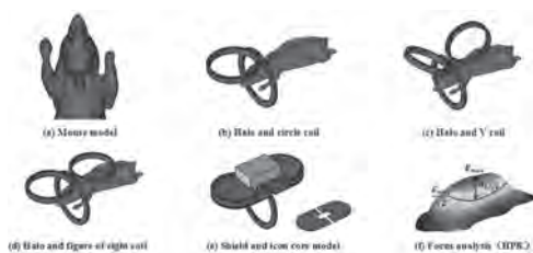
Fig.1 Mouse and coil models of this study
