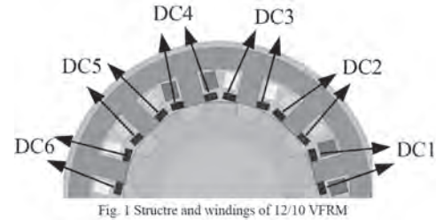
Fig. 1 Structure and windings of 12/10 VFRM
