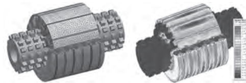
Fig.1 3D FE model of 2DoFRL-FSPM machine.
