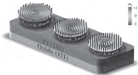
Fig.1 Sketch of modelled magnetic nanodots at selected cobalt thicknesses. The stabilized spin textures are represented by the arrows at the top of the structures. The color of the arrows represents the out-of-plane component of the magnetization. The color of the surface represents the X-component of the magnetization.
