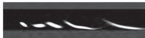
Snapshots of the time evolution of the probability density of finding a skyrmion at a certain position. The corresponding snapshot times are, from left to right, 1.5/4.5/7.8/13.5 ns. The track length is 1 mm. There are 100 pinning sites randomly distributed on the track with moderate intensity. The success probability is close to 1 (higher than when we have no granularity), with a small probability of being annihilated at the edge of the track or being trapped.
