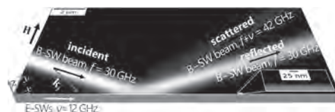
Fig. 2. Scheme of the system under investigation with the result of micromagnetic simulation performed for B-SW beam at frequency f = 30 GHz incident under the angle 60^\circ and scattered on an E-SW at v = 12 GHz. Red (at the edge), yellow and blue (beams) corresponds to presence of the SWs of frequencies v , f , and f+v , respectively. The white color denotes areas, where at least two frequencies are mixed.
