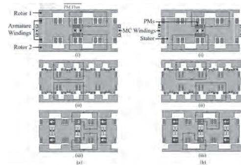
Fig. 1. Topologies and operation principles of AF-DR stator-PM motors with rotors under: (a) Aligned position: (i) DSPM motor. (ii) FRPM motor. (iii) FSPM motor. (b) Unaligned position: (i) DSPM motor. (ii) FRPM motor. (iii) FSPM motor
