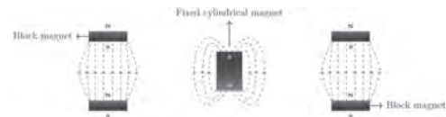
Fig 2 Cross-section of the 2-D EMVEH and magnetic flux lines between the two-ring structure(left and right) and fixed cylindrical magnet (centre).
