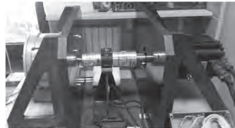
Fig. 2. Test system to investigate overhang and magnetic force during rotor moving along z-axis
