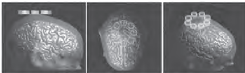
Fig. 1. Hybrid circular-solenoid coil and simulation head model in Sim4Life software.
