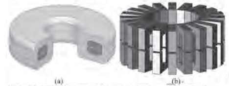
Fig. 2 CPT device 3D structure. (a) rotating transformer structure. (b) rotating transformer manufactured by ferrite pieces.
