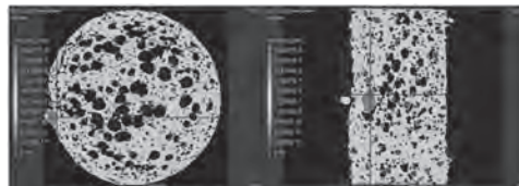
Figure 2 X-ray tomography scan performed on the produced composite filament. Iron oxide particles are highlighted with color coding by volume. The TPU matrix is colored in light gray to easily visualize the pores and iron oxide dispersions.
