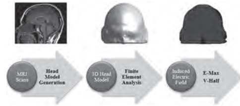
Fig. 1. Conventional Process for Induced Electric Field Estimation during TMS
