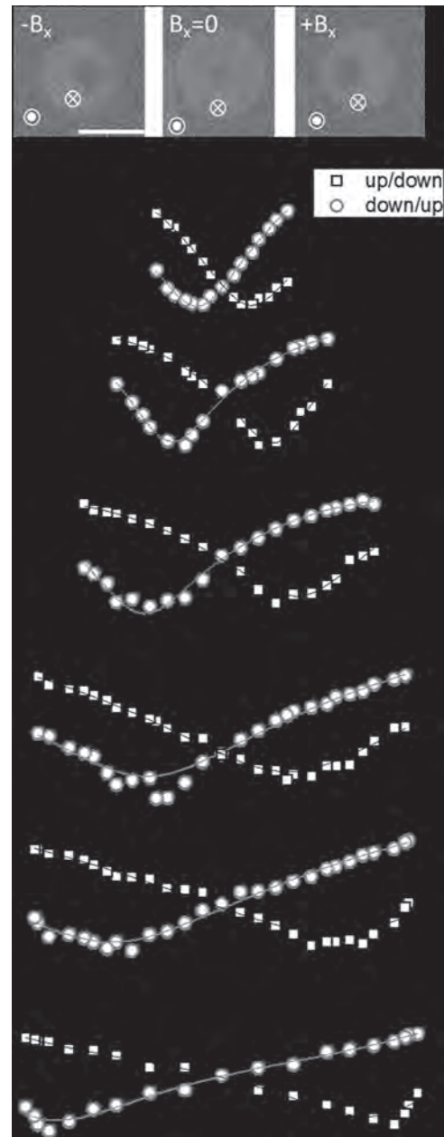
a) Expansion of Néel-type bubble in Pt|Co|Al trilayer for different external in-plane magnetic field B_x , b-g) Domain wall velocity vs. B_x for up/down and down/up DWs.
