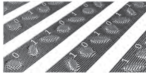
In Heusler materials the anisotropic DMI stabilizes antiskyrmions (red) and elliptically deformed skyrmions (blue). These coexisting types of topologically distinct objects may encode data as '0' and '1' bits, respectively.
