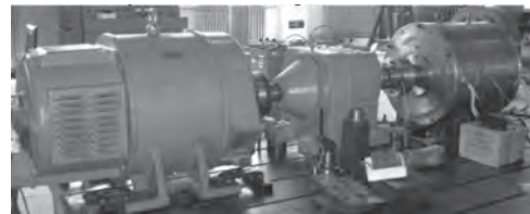
Fig. 2. Test platform of a hybrid excitation prototype.
