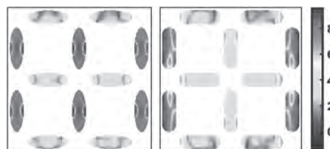
The power profile of the spin wave mode excited at ~ 6.5 GHz in S-ASI with (left) elliptical and (right) stadium-shape nanoislands at 200mT external field.
