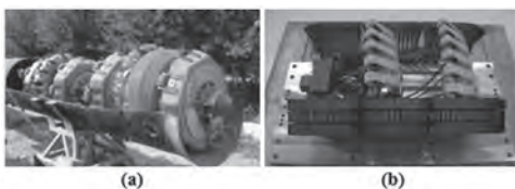
Fig. 1. The magnetic flux leakage pipe inspection devices. (a) AMFL[1] (b) CMFL[2].
