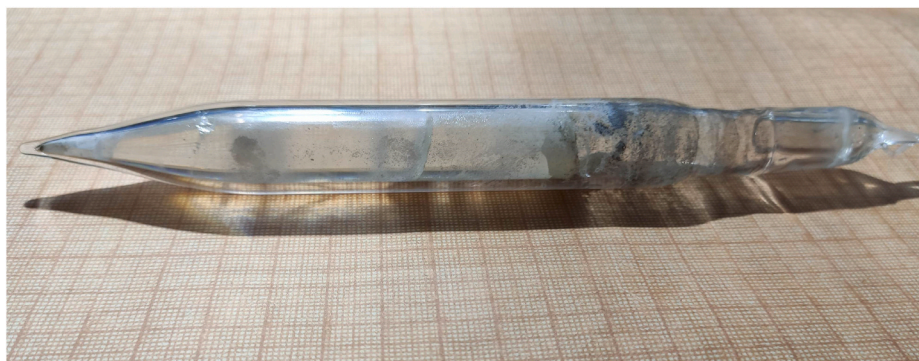
Fig. 1. A photo of the K_{0.4}Rb_{0.6}Pb_2Cl_5 single crystal applied in the present experiments.
