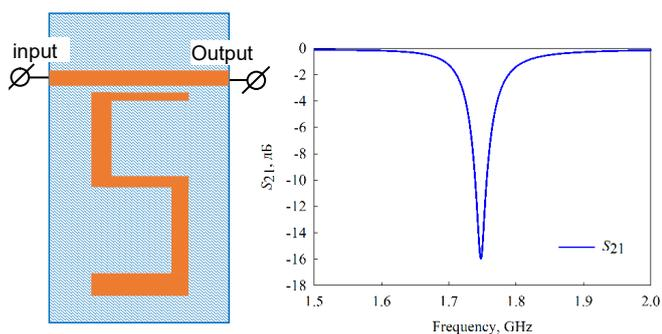
Fig. 2. Structure of one-order bandstop filter (left) and its frequency response (right)
