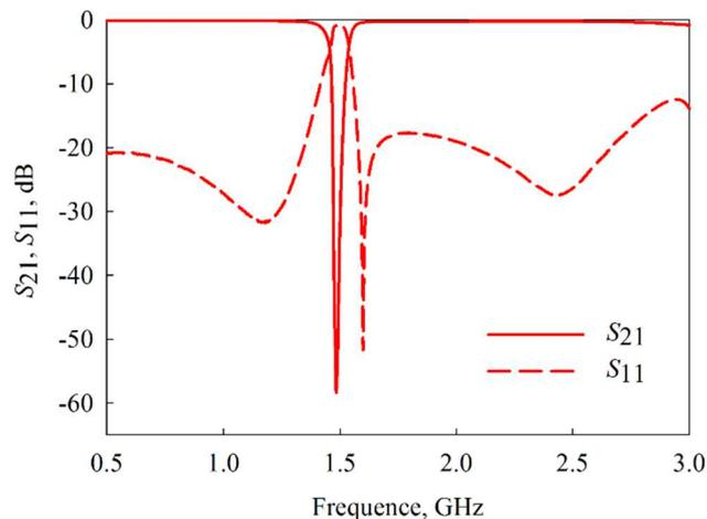
Fig.7 Measured frequency response of five-order bandstop filter in a wideband
