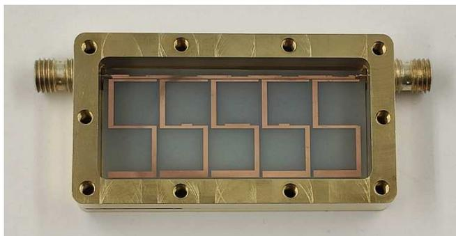
Fig. 6. Photograph of fabricated BSF
