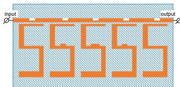
Fig. 1. Structure of a bandstop filter
