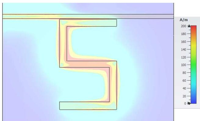
Fig. 3. Distribution of H-field in one-order bandstop filter at a resonant frequency of S-shaped resonator (1752 MHz)
