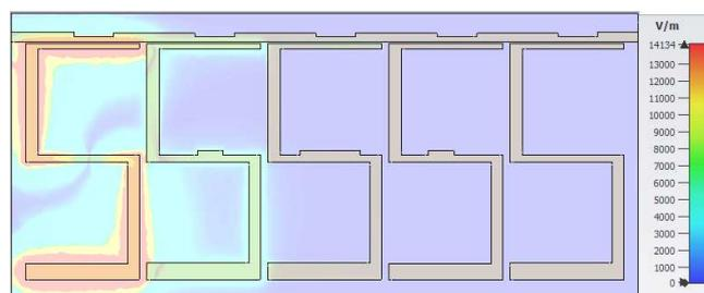
Fig. 5. Distribution of E-field in five-order bandstop filter at a central frequency of the stopband (1489 MHz)
