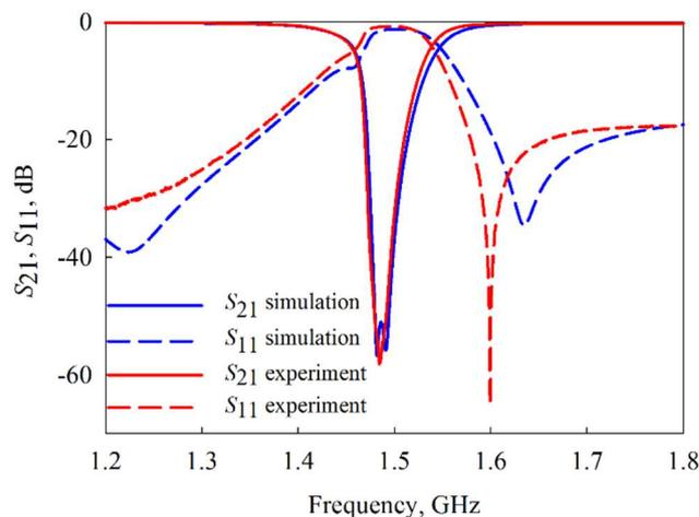
Fig. 4. Frequency response of the five-order bandstop filter
