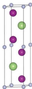
Fig. 1 Crystal structure of M_2AX phase. M, A, and X atoms are shown by purple, green, and grey balls, correspondingly.
