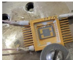
Fig. 1. Photo of diode structure in the chip package.
