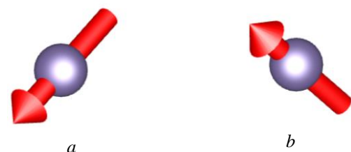
Fig. 2. Magnetization direction with negative (a) and with positive external pressure (b) in the Ge {105} system with hole qubit.
