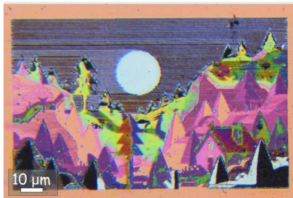
Fig. 2. Large-scale ( 120 \times 60 \mu\text{m}^2 ) structural color image with the of produced by direct laser printing on MIM sandwich structure. 14 different color tones varied by tuning the applied pulse energy/period were used. The image was captured with optical microscope at \text{NA}=0.3 in reflection mode.
