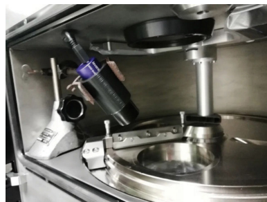
Figure 1. Camera Levenhuk M500 Base in the built chamber of the 3D printer.
