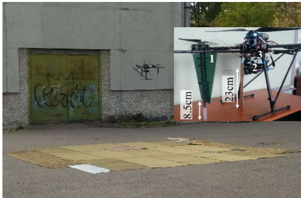
Fig. 3. UAV over a brass mesh during antenna calibration. 1) LPDA, 2) LIDAR-Lite v3, 3) VNA CABAN R60.
