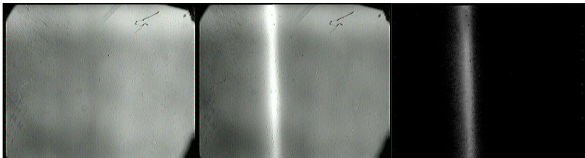
Figure 1. MO Image of the defective area: a) in the position of phase 1, b) in the position of phase 2, c) the result of subtracting two phases.
