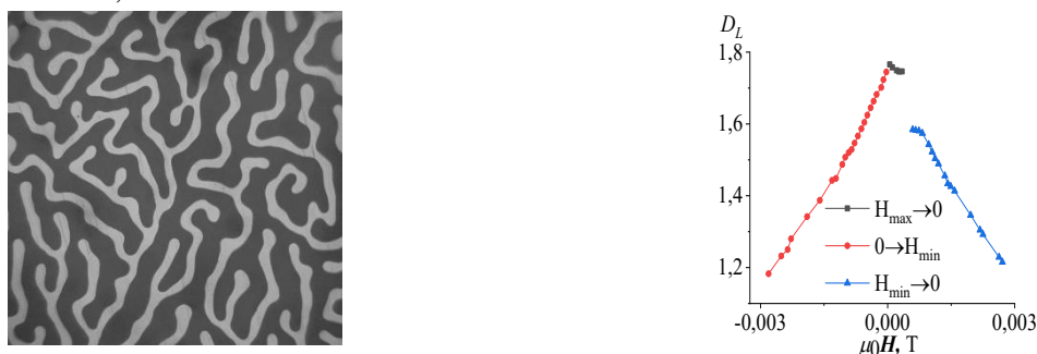
Fig. 1. Magneto-optical image of the domain structure for the FG film (\text{GdBiLuSm})_3(\text{FeGa})_5\text{O}_{12} (left) and field dependence of the FD value (right)
