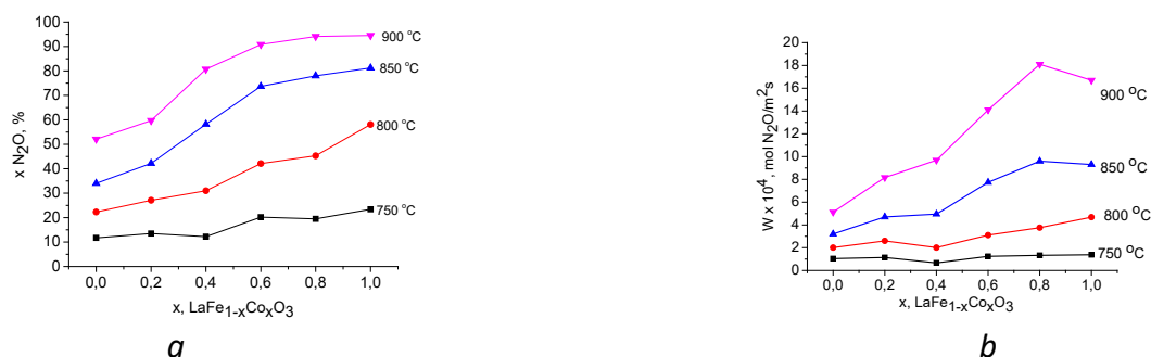
Figure. Dependence of conversion (a) and rate of decomposition reaction (b) of nitrous oxide on the composition for perovskites \text{LaFe}_{1-x}\text{Co}_x\text{O}_3 .
