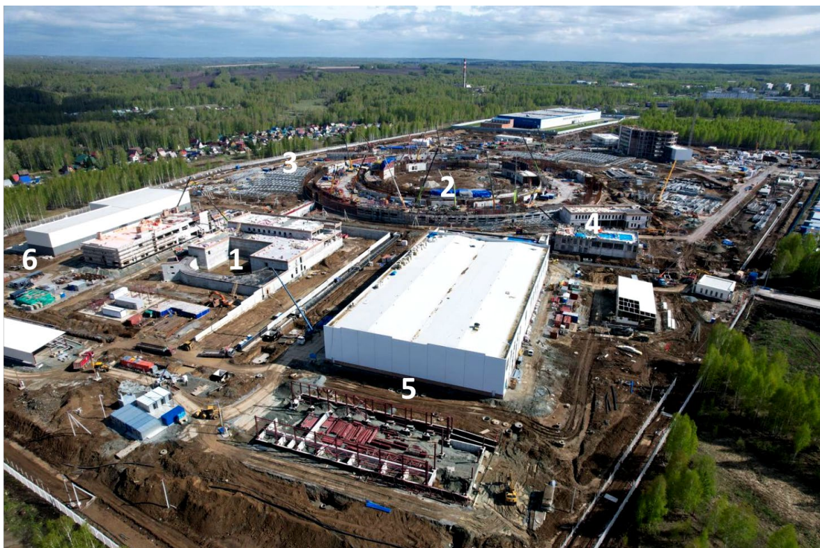
Fig. 1. An aerial view of the SKIF construction site as of May, 2024: 1 – injector building, 2 – main storage ring building, 3 – beamline 1-3 “Fast processes” external building, 4 – beamline 1-5 “Hard X-ray diagnostics” external building, 5 – building of stands and testing facilities, 6- building of engineering facilities
