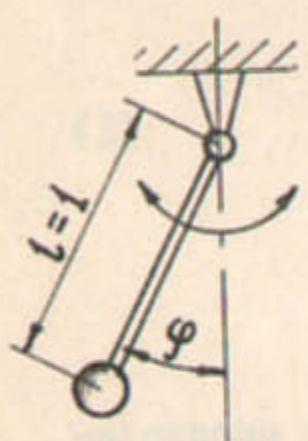
$$\text{I} \quad \frac{v_0 w}{l} \gg 1 \\ g = \frac{v_0^2}{l} \omega_l \sin \omega t, \quad \varphi \rightarrow \omega \frac{z}{l}.$$
