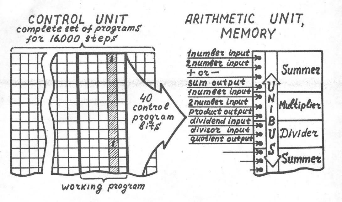
Fig. 2 The principle of the processor operation.
