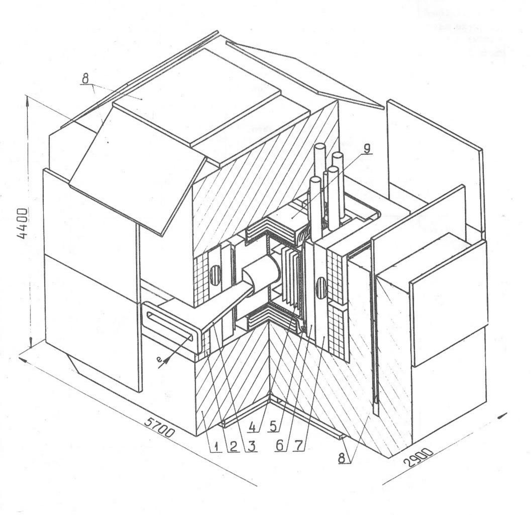
Fig. 1 Magnetic detector MD-1. 1 - yoke, 2 - copper winding, 3 - vacuum chamber, 4 - coordinate chambers, 5 - scintillation counters, 6 - gas Ĉerenkov counter, 7,9 - shower-range chambers, 8 - muon chambers.
