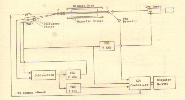
Fig. 2. The scheme of the experiment. P-prism polarizer,
