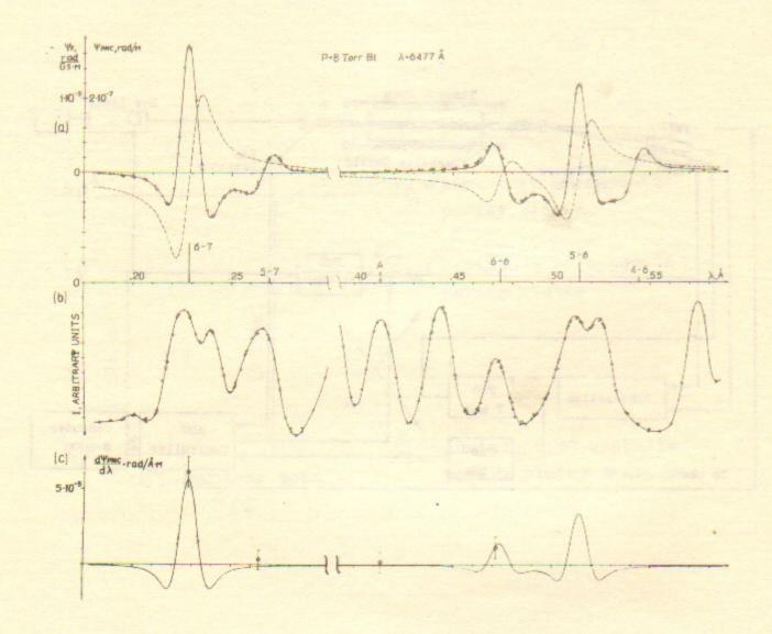
Fig. 3. a - Dashed line - the theoretical prediction for PNC optical rotation of bismuth vapor, solid line/3/. the calculated Faraday rotation; b - observed absorption spectrum; c - the calculated curve and the results of the measurements.
