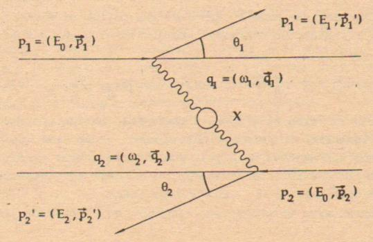
The electron and positron radiate virtual photons which produce a C-even state X. Due to the photon propagators of this diagram the cross section is determined by small invariant masses of photons  $q_1^2 = -Q_1^2 = (p_1 - p_1')^2$ . In other words most of the photons are emitted at small angles and are quasi-real.
